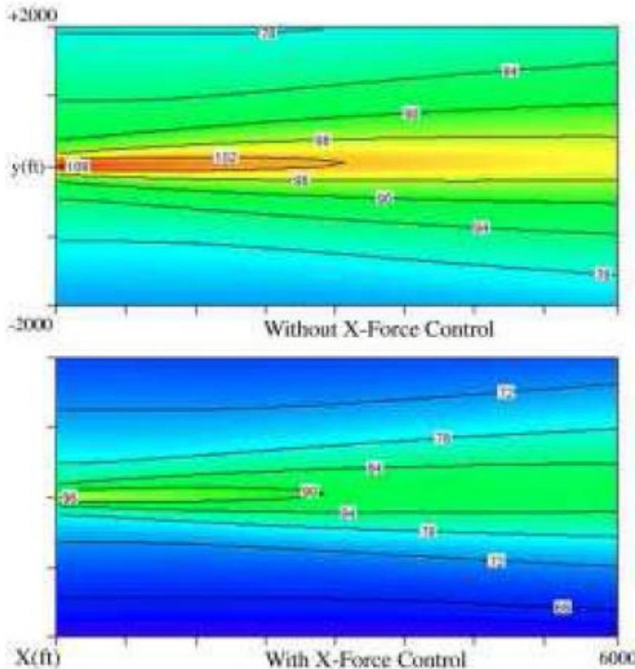
Predicted Ground Noise without / with X-Force Control at 3° Approach Angle<sup>12</sup>
