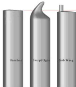
Figure 5<sup>4</sup>: Rotor Blade Tips
