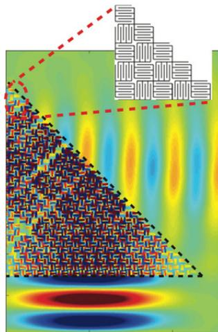
Figure 8: Meta-material Acoustic Blanket
