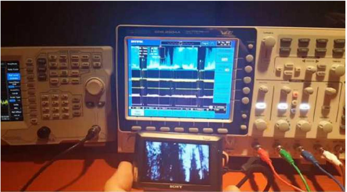
Oscilloscope capture of camera signals from the Sony video camera .
